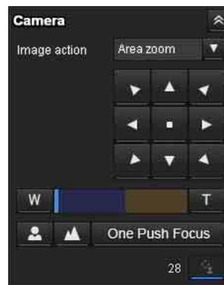
On this panel, you can control the pan/tilt/home position of the camera, adjust the zoom and switch focus mode (page 25). In addition, you can obtain authority to operate the camera when the exclusive control mode is on.
